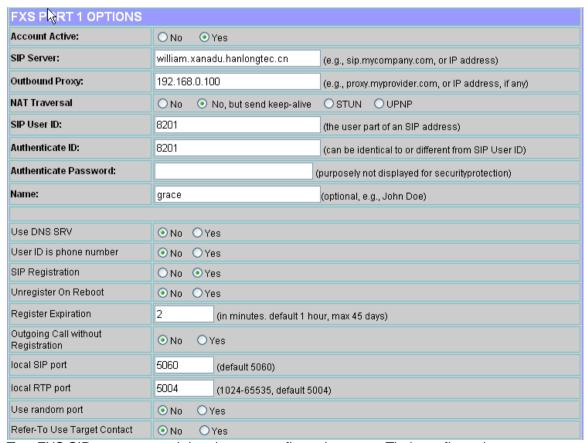
Two FXS SIP accounts each has its own configuration page. Their configurations are identical. The following is a screen shot of FXS Port 1 Account settings.
