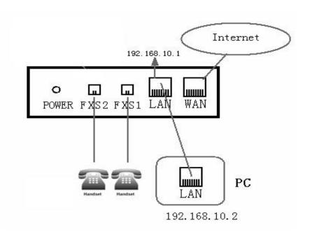
A2 two-port gateway with two network interface itself: WAN port and LAN port, you can use the Internet connection into the WAN port or LAN port. Read the manual carefully of "Safety" before inserting the power
