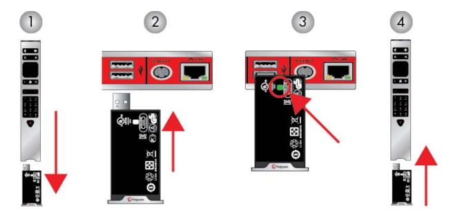
If you have a RealPresence Group 700 system, you can also recharge the battery using the USB port on the front of the system.
