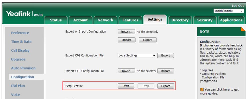
2. Click **Start** in the **Pcap Feature** field to start capturing signal traffic.
