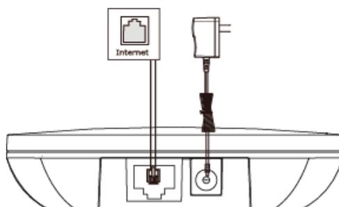
**Note** The base station should be used with original power adapter (5V/600mA) only. The use of the third-party power adapter may cause the damage to the phone.
