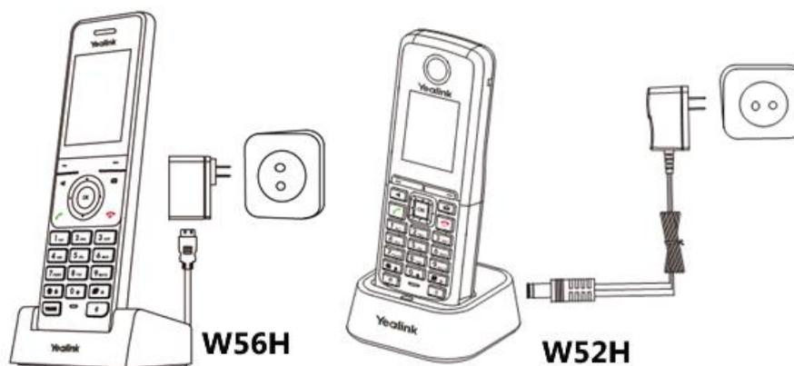
**Note** The handset should be used with Yealink original power adapter (5V/600mA) only. The use of third-party power adapter may cause the damage to the phone.
