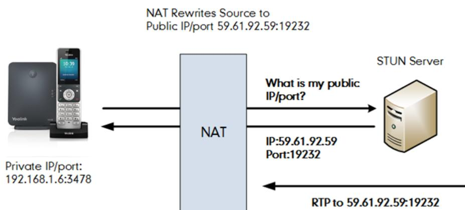
Capture packets after you enable the STUN feature, you can find that the IP phone sends Binding Request to the STUN server, and then mapped IP address and port is placed in the Binding Response: Binding Success Response MAPPED-ADDRESS: 59.61.92.59:19232.
