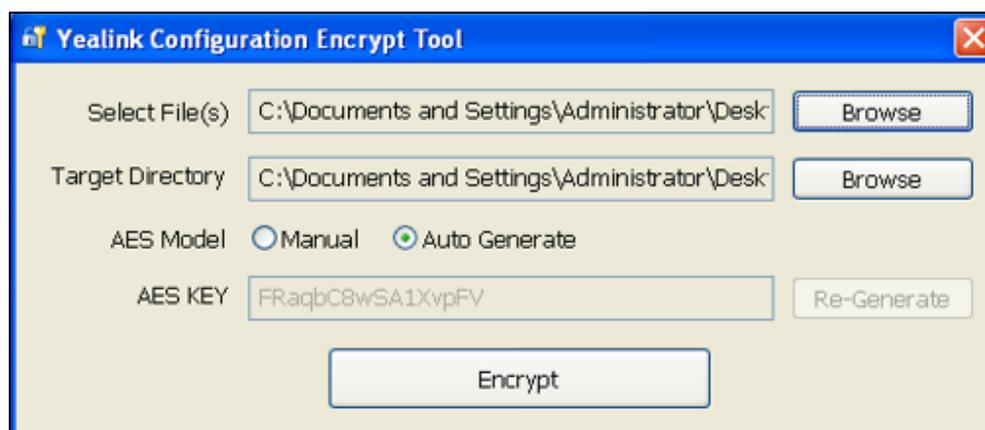
When you start the application tool, a file folder named "Encrypted" is created automatically in the directory where the application tool is located.
