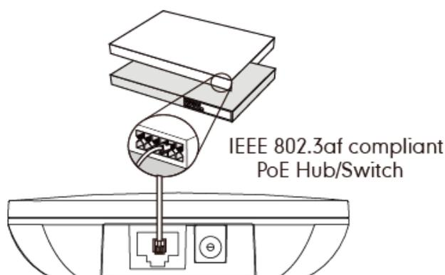
**Note** If in-line power is provided, you don't need to connect the AC adapter. Make sure the switch/hub is PoE compliant.
