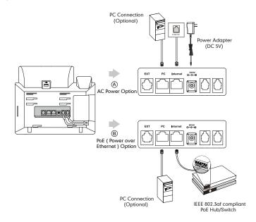
Note: If inline power (PoE) is provided, you don't need to connect the power adapter. Make sure the Ethernet cable and hub/switch are PoE compliant.
