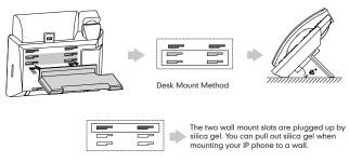
Note: For more information on how to mount the IP phone to a wall, refer to Yealink Wall Mount Quick Installation Guide for SIP-T4X IP Phones.
