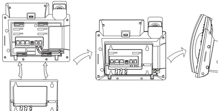
**Note** The wall mount bracket should be purchased separately. For more information on how to attach the wall mount bracket, refer to *Yealink Wall Mount Quick Installation Guide for T4X IP Phones*.
