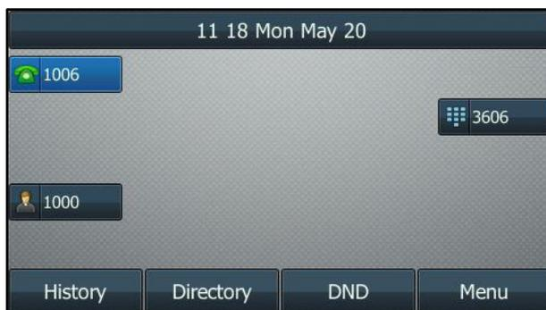
When you assign functionality to line key located in line key 11-27, the label of the line key 10-18 are indicated on the second page, and the labels of the line key 19-27 are indicated on the third page. The right bottom line key is used to switch pages. The following figure shows an example:
