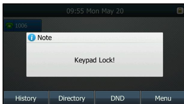
You can configure the interval (in seconds) to automatically lock the keypad instead of long pressing
