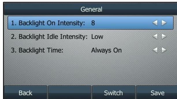
2. Press  $\leftarrow$  or  $\rightarrow$ , or the **Switch** soft key to select the desired level from the **Backlight On Intensity** field.
