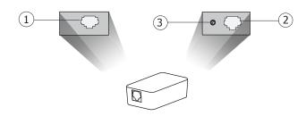
Port ①: Connect with the IP Phone EXT port or Expansion Module port (expansion module connected to the phone) through RJ12 cord.
