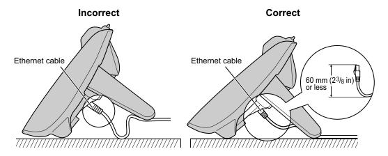
Use a straight CAT 5 (or higher) Ethernet cable (not included) that is 6.5 mm (<sup>1</sup>/<sub>4</sub> in) in diameter or less.
