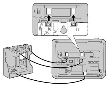
2. Fasten the wall mounting adaptor to the base with 1 screw. (Recommended torque: 0.4 N·m [4.08 kgf·cm/ 3.54 lbf·in] to 0.6 N·m [6.12 kgf·cm/5.31 lbf·in])
