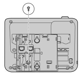
**3.** Connect the cables to the unit, and run the cables through the wall mounting adaptor, as shown in the illustration below.
