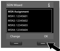
After the MSNs have been successfully assigned, a list containing the MSNs is displayed.
