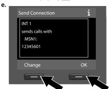
The send connection currently set for the base is displayed: MSN1 for connection to the ISDN and Fixed Line for connection of the Gigaset DX800A all in one to the analogue fixed line.
