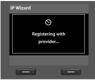
Once you have made all the necessary entries, the VoIP wizard tries to register the base with the VoIP provider.
