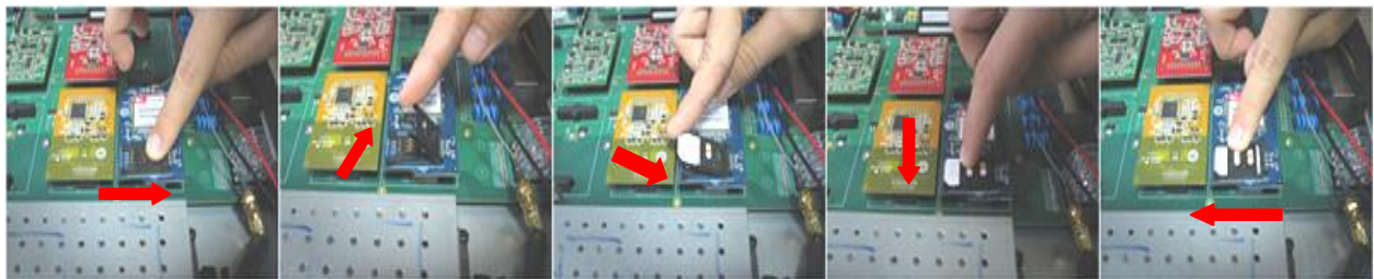
Figure 3-2 Inserting the SIM Card
