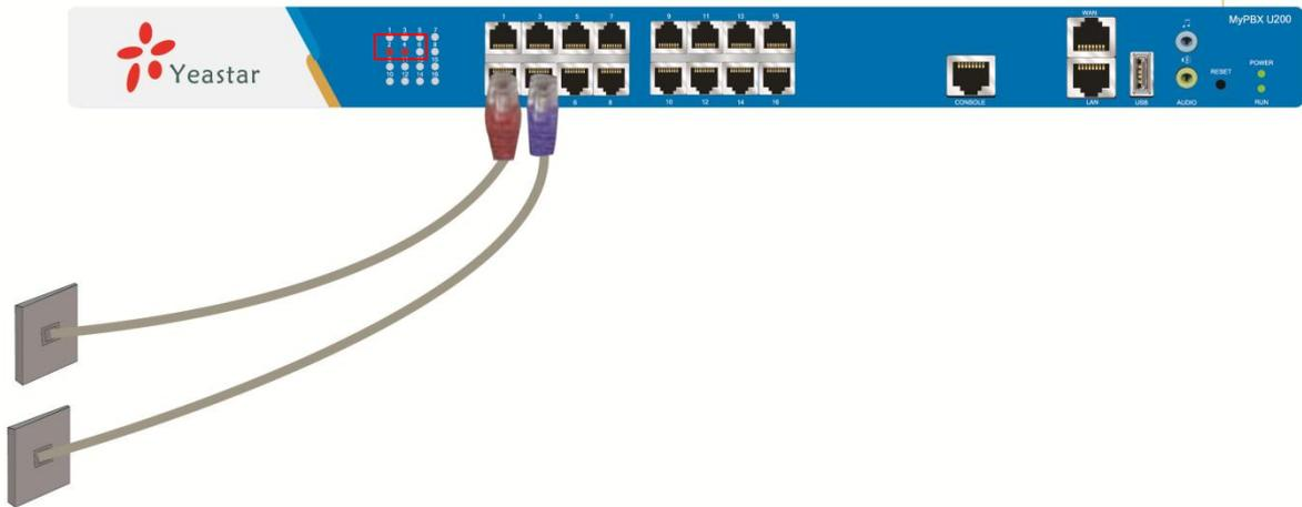
Figure 3-1 Connection of FXO ports
