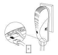
phone cable to a jack wired for a standard analog phone line.
