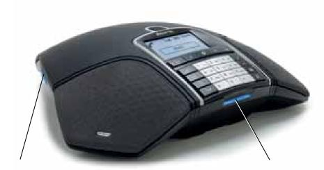
The **Konftel 300Wx** is a battery-driven wireless conference phone that can be connected to DECT systems, mobile phones or PCs. It can be connected to a Konftel DECT base station or any GAP/CAT-iq-compatible DECT system.
