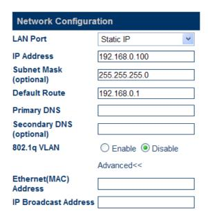
The default setting of GoIP1 is **Static IP** with IP address "192.168.0.100" and **Subnet Mask** "255.255.255.0". However, **Default Route**, **Primary DNS**, and **Secondary DNS** (optional) must be manually entered according to your network configuration.
