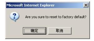
Click OK. All the parameters of the gateway will be cleared and the gateway will automatically restart. After the gateway is restarted, all the settings restore to the factory default settings. This feature can be completed by using the asterisk command. For details about this operation, see the
