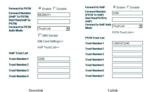
The setting is as follows: Select "Forward to PSTN Authentication Mode" > "Trust List Authentication". Click the "VoIP Trust Number List", and the VoIP Trust Number List is displayed (Maximum 15 trust numbers can be entered). Enter the trust VoIP number in trust number sequence.
