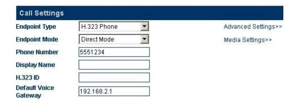
Under this mode, the GoIP operates in the point-to-point status. The setting parameters are as
