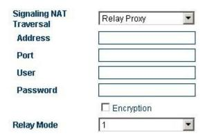
The trunk agent protocol supports encryption on communications over the gateway. This feature needs the support of the server developed by DBL Technology.
