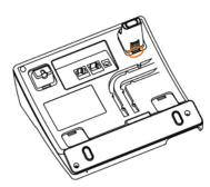
B. Press the other plate into the slot in accordance with the direction of the arrow
