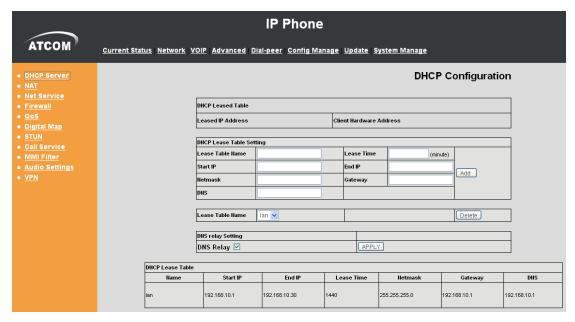
DHCP Leased Table: IP-MAC mapping table. If the LAN port of the phone connects to a device, this table will show the IP and MAC address of this device. Leased IP Address: the IP address which is assigned.
