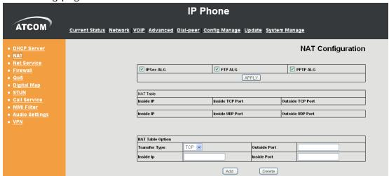
IPSec ALG: It is an encryption technology. Select it to enable IPSec ALG, the default is enable.
