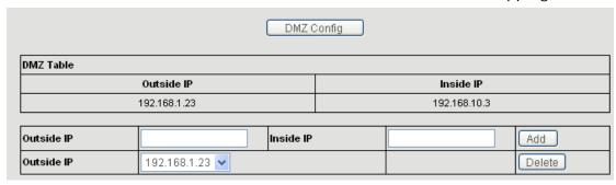
DMZ Table: Shows the outside WAN port IP address and the inside LAN port IP address.
