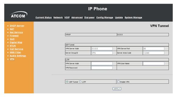
this page is VPN setting page , the IP phone support the VPN with UDP and L2TP protocol .The parameters is as below.
