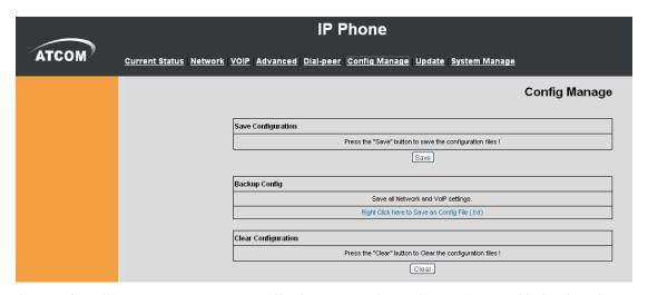
**Save Config:** you can save all changes of configurations. Click the Save button, all changes of configuration will be saved, and be effective immediately. **Backup Config:** Right clicks on "Right click here..." and select "Save Target As...." then you will save the config file in .txt format
