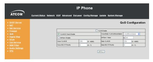
VLAN Enable: Before select it to enable VLAN, you need enable Bridge mode in LAN config.
