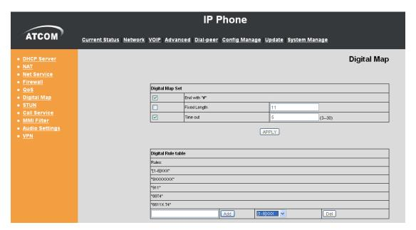
Digit map is a set of rules to determine when the user has finished dialing. AT620P support below digital map:
