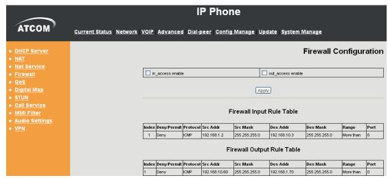
in\_access enable: Select it to Enable in\_ access rule;out\_access enable: Select it to Enable out\_ access rule
