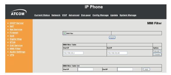
User could make some device own IP, which is pre-specified, access to the MMI of the phone to config and manage the phone.
