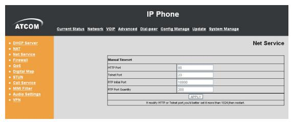
**HTTP Port:** set web browser port, the default is 80 port, if you want to enhance system safety, you'd better change it into non-80 standard port; Example: The IP address is 192.168.10.88. and the port value is 6090, the accessing address is <a href="http://192.168.10.88:6090">http://192.168.10.88:6090</a>
