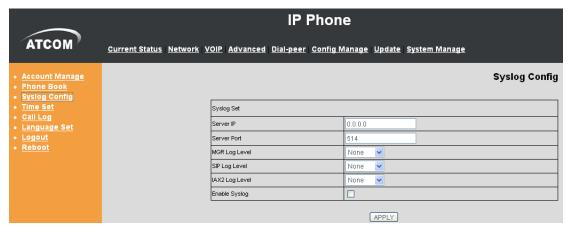
Syslog is a protocol which is used to record the log messages with client/server mechanism.
