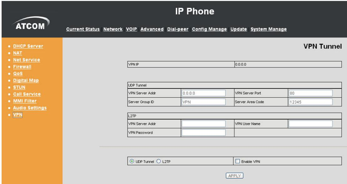
this page is VPN setting page , the IP phone support the VPN with UDP and L2TP protocol .The parameters is as below.
