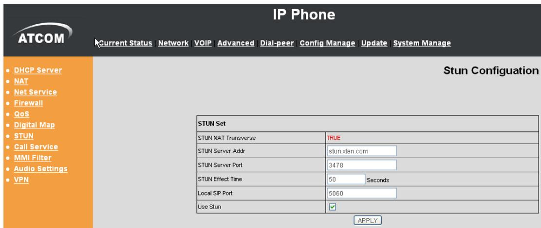
The screenshot shows the 'IP Phone' configuration interface with a sidebar menu on the left containing options like DHCP Server, NAT, Net Service, Firewall, QoS, Digital Map, STUN, Call Service, MMI Filter, Audio Settings, and VPN. The main content area is titled 'Stun Configuration' and contains a table for 'STUN Set' with the following fields:
