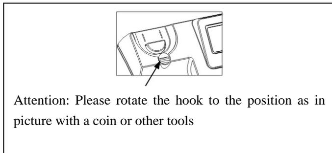
D、 Disassemble the feet way:
