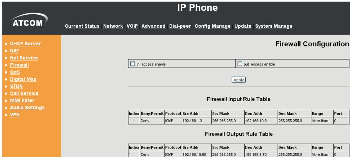
The screenshot shows the 'IP Phone' configuration interface with a 'Firewall Configuration' section. On the left is a navigation menu with items like DHCP Server, NAT, Net Service, Firewall, QoS, Digital Map, STUN, Call Service, MMI Filter, Audio Settings, and VPN. The main area contains two checkboxes for 'in\_access enable' and 'out\_access enable', an 'Apply' button, and two tables: 'Firewall Input Rule Table' and 'Firewall Output Rule Table'.
