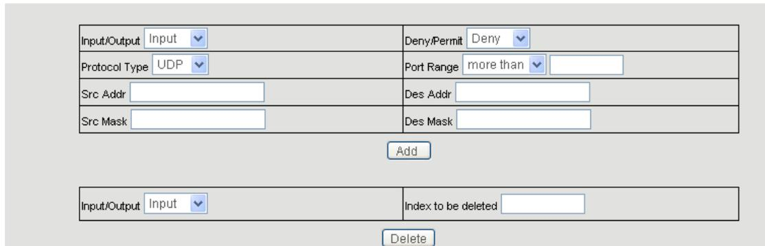
The screenshot shows the configuration form for adding or deleting a firewall rule. It includes fields for Input/Output, Deny/Permit, Protocol Type, Port Range, Src Addr, Des Addr, Src Mask, and Des Mask. There are 'Add' and 'Delete' buttons.
