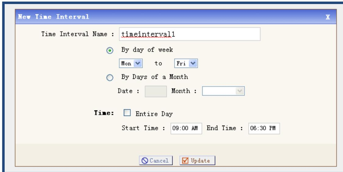
**Time Interval Name:** a unique label to help you identify the time interval when listed in incoming calling rules. I set up timeinterval1 as time interval name.
