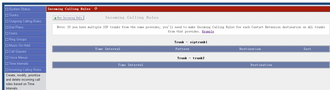
Click on **New Incoming Rule** button on the illustration above, the following screen is where you create and set up time interval:
