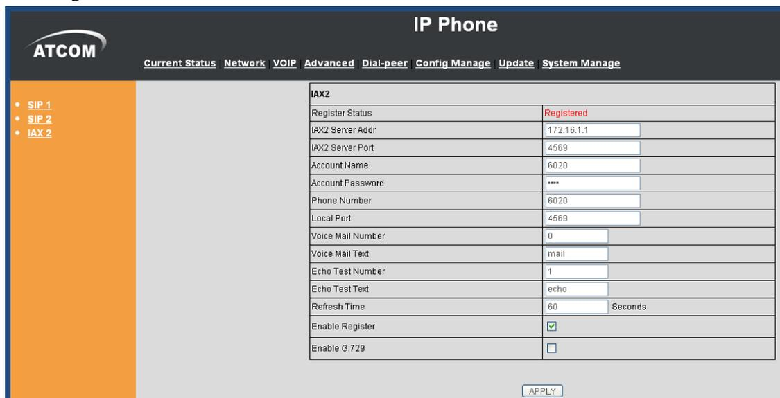
The screenshot shows the 'IP Phone' configuration page with the 'VOIP' tab selected and the 'IAX2' sub-tab active. The left sidebar has 'SIP 1', 'SIP 2', and 'IAX 2' options. The main content area displays the following configuration details:
