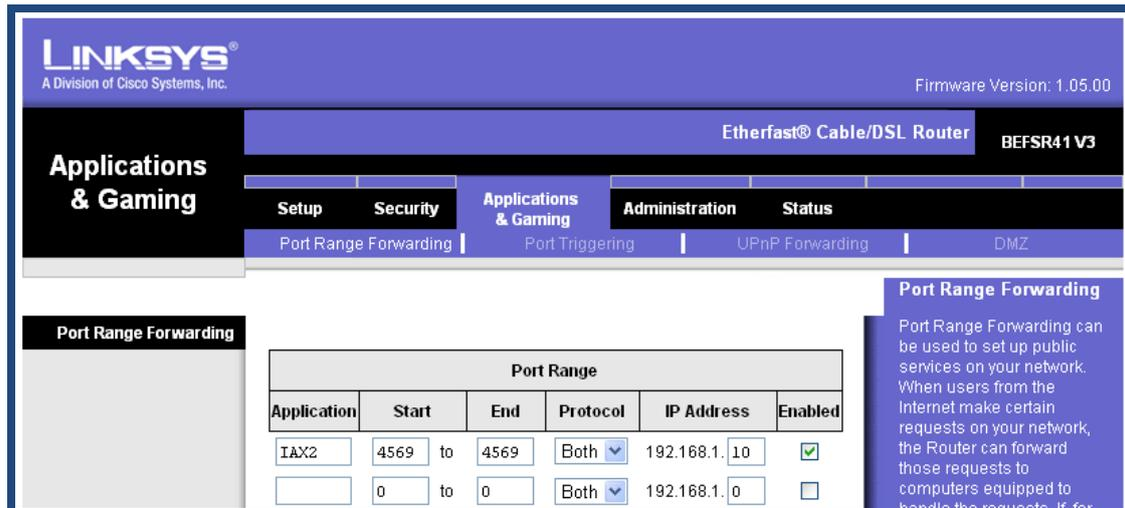
The user 6020 uses IAX2, the port number is 4569, 192.168.1.10 is the IP address of IP01.
