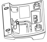
$C_{\Sigma}$  Repeat A and B. It is the picture of wall mounting after fixing the two feet below:
