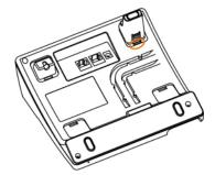
B、 Press the other plate into the slot in accordance with the direction of the arrow
