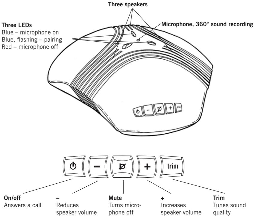
Konftel 60W is a conference unit for connecting to existing fixed system telephones, DECT telephones, cell phones or computers, with a cable or wireless connection via Bluetooth. Konftel 60W has an omnidirectional, highly-sensitive microphone and three speakers which, together with Konftel's OmniSound® provide optimal sound quality and maximum reduction of room echo, even when the person speaking is standing at a slight distance from the unit.
